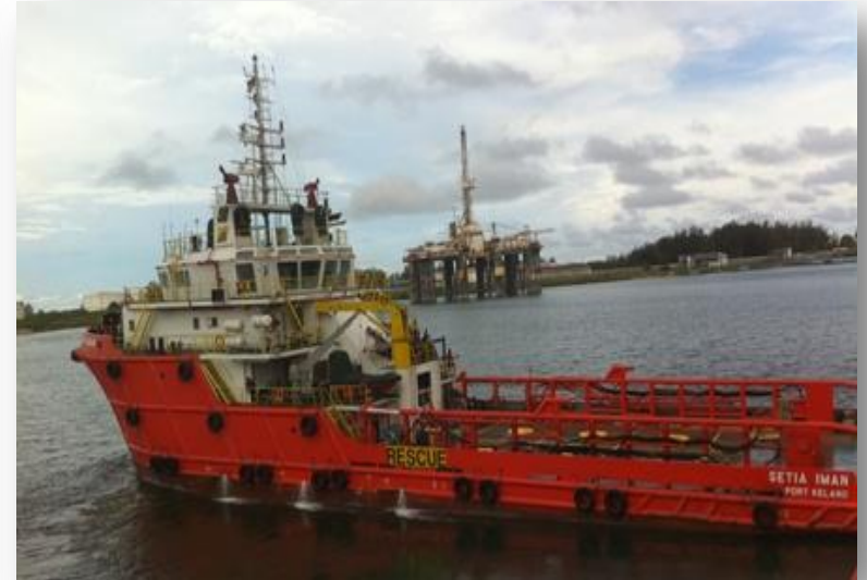
TH ALAM MANAGEMENT M V SETIA IMAN - ANCHOR HANDLING TUG SUPPLY (AHTS) VESSEL (DP 1)
