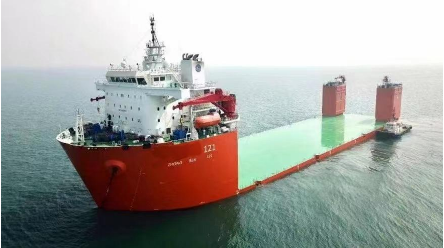
Multi-purpose Offshore vessel, DP2, 2x4500kw for main propulsion and 4X2400kw thrusters Owner: Ministry of Transport of People's Republic of China
